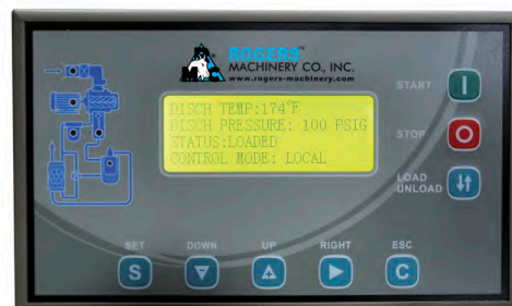
KI Control Panel
